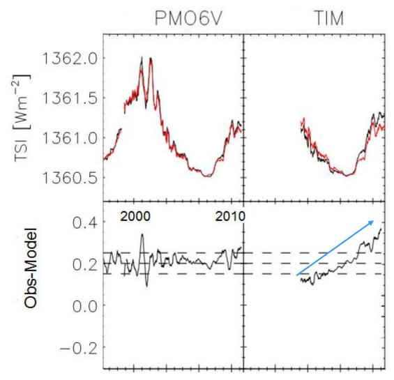
The Yeo et al. model reconstructs TSI (red curves) from MDI and HMI magnetograms. TIM has the least noise but seems to be drifting (upwards)
