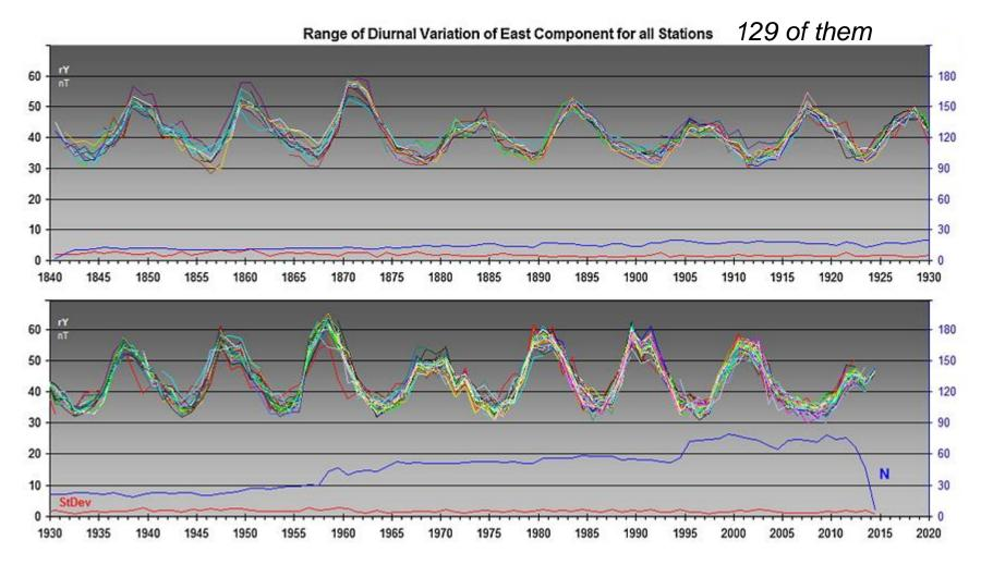
We plot the yearly average range to remove the effect of changing solar zenith angle through the seasons. What remains is the solar cycle modulation. The blue curve shows the number of stations
