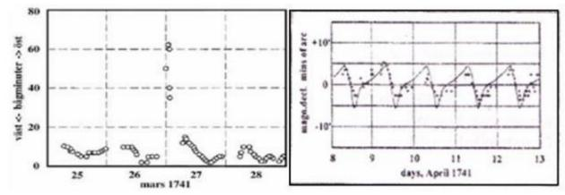
Right: Hjorter's measurements of the magnetic declination at Uppsala during April 8-12, 1741 (old style). The curve shows the average variation of the magnetic declination during April 1997 at nearby Lovö (Sweden).
