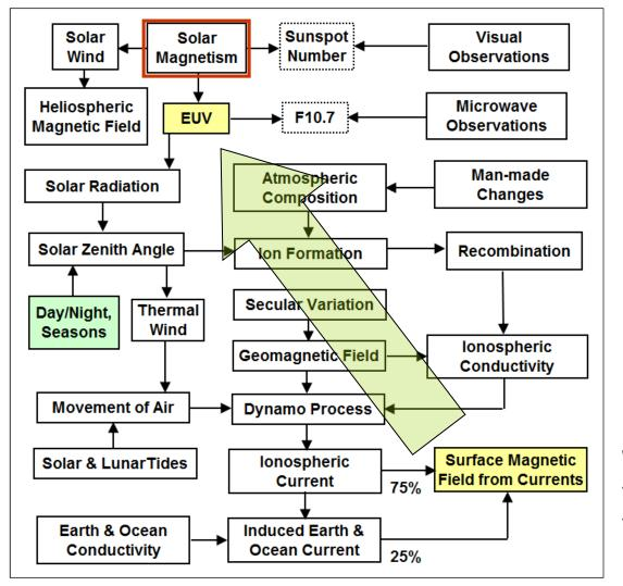
The EUV causes an observable variation of the geomagnetic field at the surface through a complex chain of physical connections.
