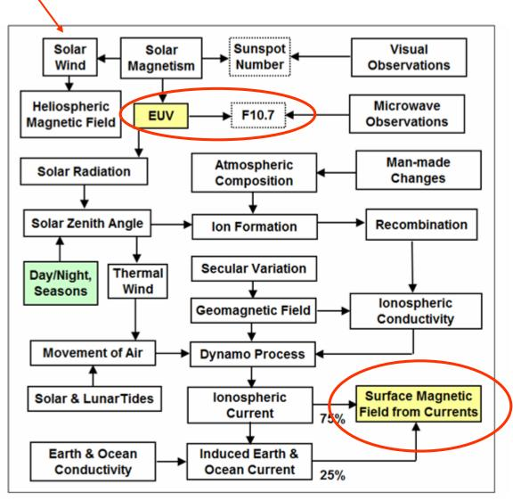
The EUV causes an observable variation of the geomagnetic field at the surface through a complex chain of physical connections.
