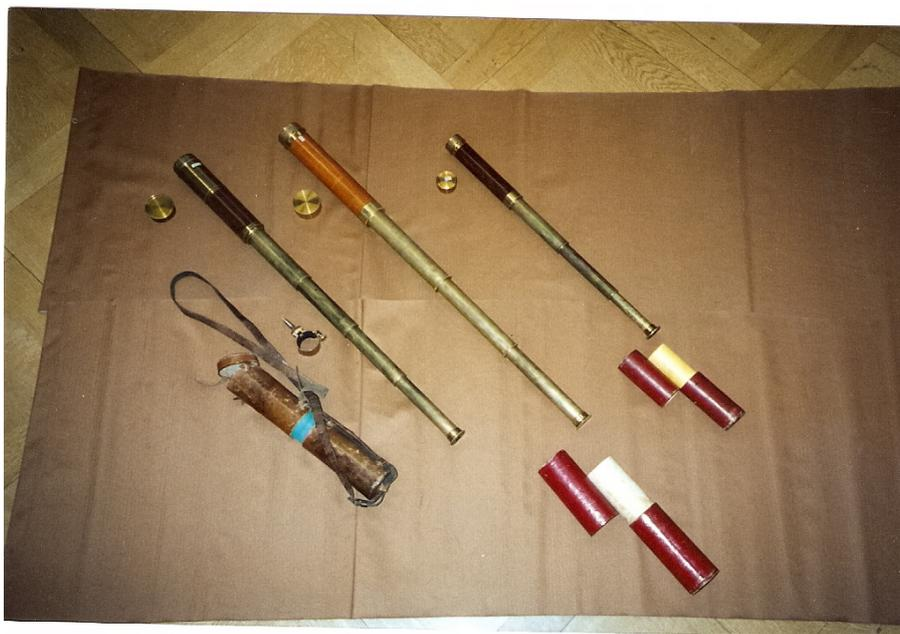
**Figure 9.** (Left) the 40/600mm hand-held refractors (at magnification 40) used by Wolf increasingly from 1860 and exclusively from 1870 for direct visual observation. The left-most is the ‘Pariser 2-füßer’ with which most of the work was done.
