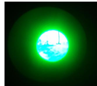
Littrow lens contamination (enhanced) seen from 75' in spring 2017 (above). Cleaned lens on May 17, 2017 (below)
