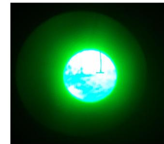
Littrow lens contamination (enhanced) seen from 75' in spring 2017 (above). Cleaned lens on May 17, 2017 (below)
