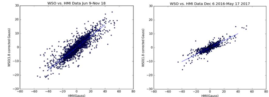
We synthesize the 195 WSO pixels for each magnetogram during normal (441) and reduced-sensitivity (99) time intervals from the nearest 720s 4k\*4k HMI image. We account for orientation and location of each pixel. This gives us many more measurements of the sensitivity difference than the daily mean field. We found WSO/HMI ratios of 0.454 and 0.293 during normal and reduced sensitivity times.
