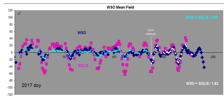
The Mean Field after the cleaning [marked with white triangles] again follow the SOLIS measurements with the usual factor of ~2 instead of the ~4 when the lens was dirty.
