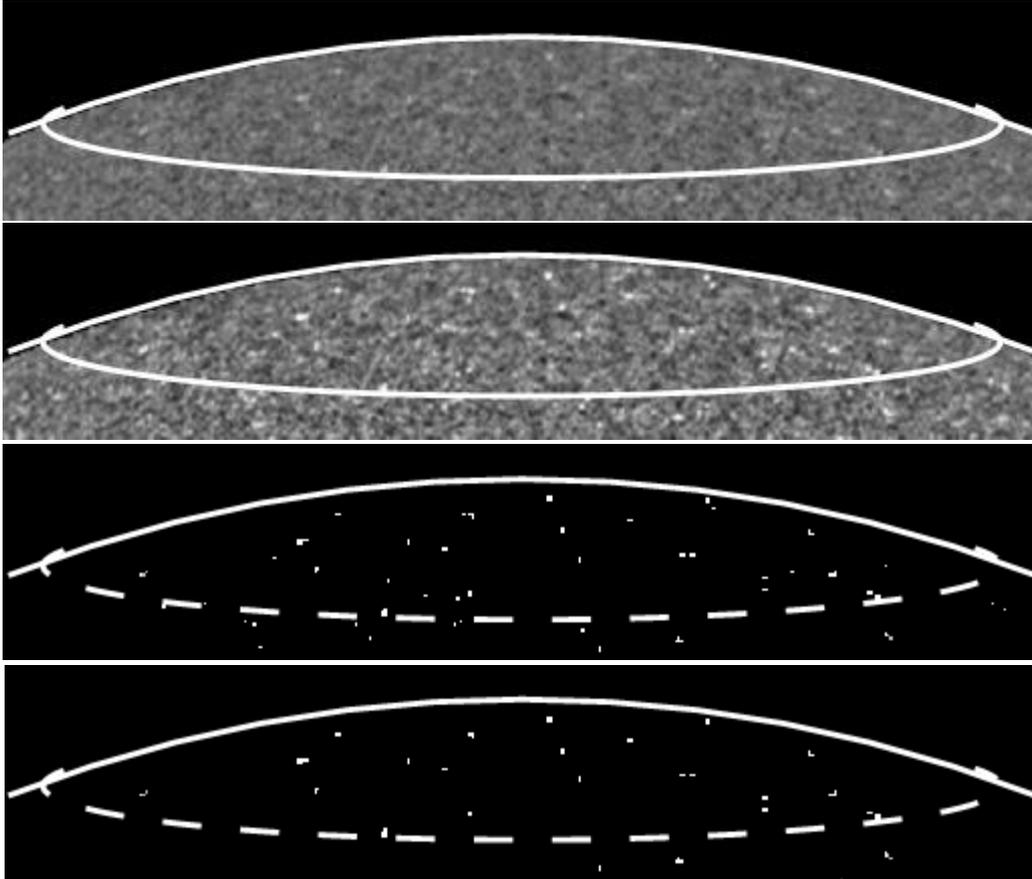
1: Perform 'gamma scaling' of the image to enhance contrast using the expression  $f(x) = 100x^\gamma$  where  $\gamma = 15$  is the enhancement exponent
