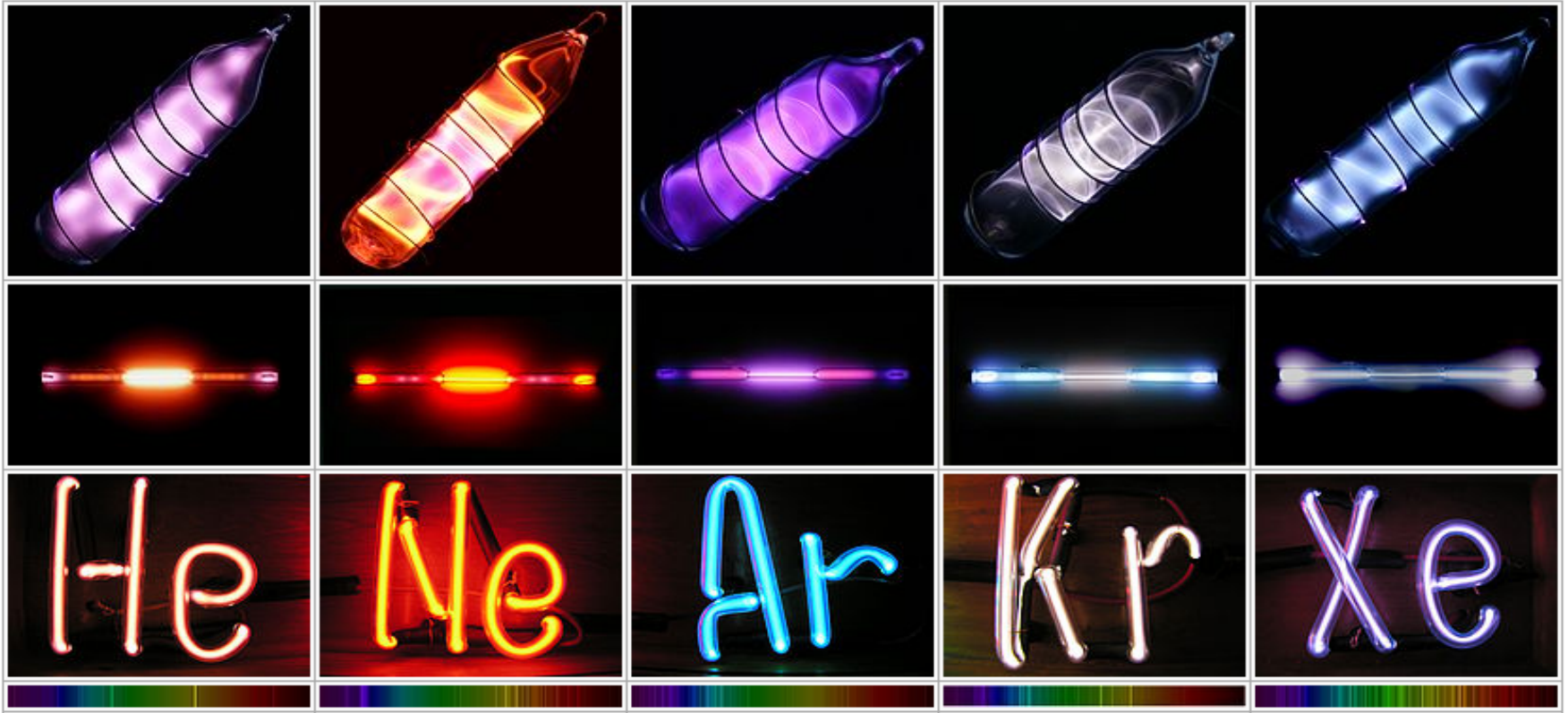
Colors and spectra (bottom row) of electric discharge in pure noble gases
