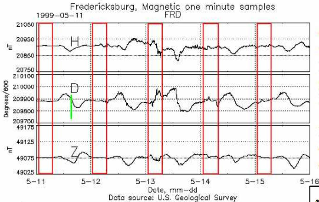
Calculating the variation (sum of unsigned differences from one hour to the next) of the field during the night hours [red boxes] from simple hourly means (the Interhourly Variation) gives us a quantity that correlates with  $BV^2$  in the solar wind
