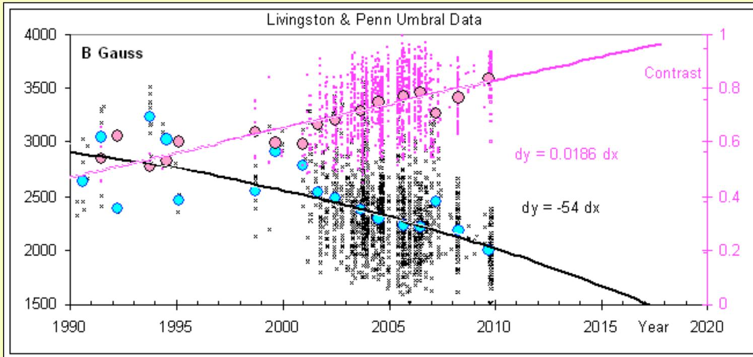
Routine IR photometry and Zeeman measurements from KPNO by W. Livingston and M. Penn at 1564.8 nm
