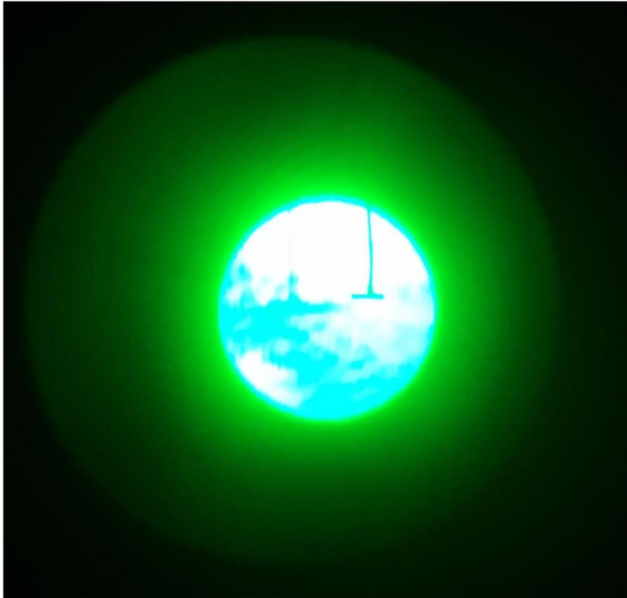
There is a lens in front of the grating in the pit. The lens makes the incoming light rays parallel before they hit the grating and collimates the dispersed light to focus at the sensors in the observing room. Todd Hoeksema pointed his iPhone at the lens and imaged it. The image showed that the lens was very dirty. 9
