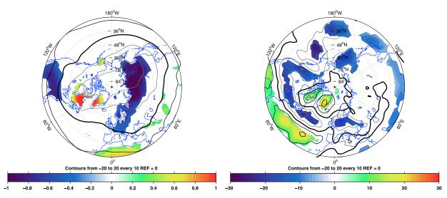
**Figure 3.** (left) The regression of the 850mb temperature on the NINO3, NAO and NINO-NAO indices (color) with the mean 850mb temperature contoured (0°*C* isotherm bold, negative contours dashed), and (right) the regression of 300mb submonthly transient eddy meridional velocity variance,  $v^2$ , all for the December through March seasonal mean. Patterns are plotted only where significant at the 5% level. Units are °*C* for temperature and  $m^2s^{-2}$  for velocity variance.
