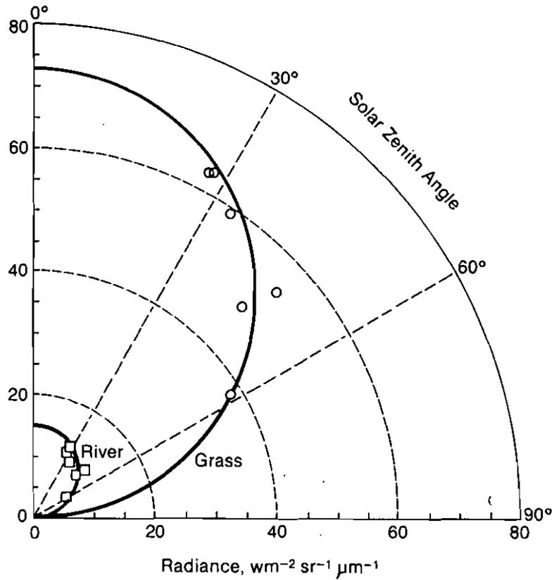
Figure 1. Raw radiances from grass and water. Heavy dark lines are radiances which satisfy the Lambertian assumption.
