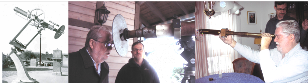
Figure 2. Left: the 80 mm Fraunhofer refractor used since 1855 by Wolf and successors until 1996. At the eye piece can be seen the Merz polarizing helioscope employed to reduce light intensity to comfortable levels. Center: the same telescope in use today by Thomas Friedli (person at right). Right: the 37 mm portable telescope used by Wolf since the mid 1860s.
