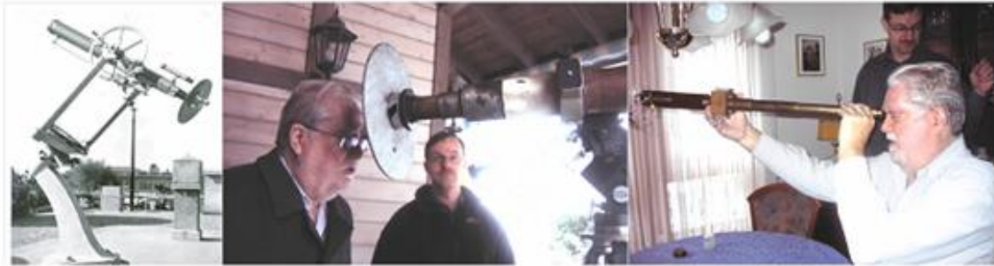
Figure 4: (Left) The 80 mm aperture (magnification X64) refractor used mostly by Wolf’s assistants at the Zürich Observatory since 1863, designed by Joseph Fraunhofer and manufactured in 1822 at the Fraunhofer factory by his assistant Georg Merz. (Middle) The telescope still exists and is being used daily by Thomas Friedli (person at center). (Right) One of several small, portable, handheld telescopes (40 mm aperture, magnification X20) used by Wolf almost exclusively from 1859 on, and still in occasional use today.
